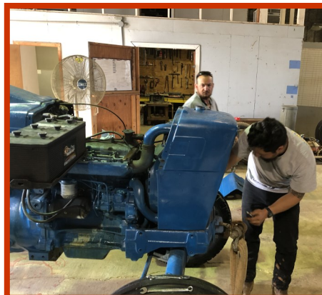
2ND YEAR APPRENTICE STEVEN MAGGARD WITH 1ST YEAR APPRENTICE WILFREDO CASTRO WORKING ON TRACTOR, REPLACING WATER PUMP
